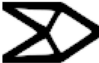
Figure 6. Optimum layout by SIMP and FEM [33]
