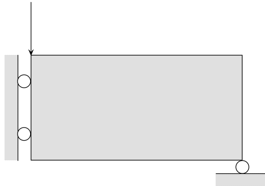
Figure 1. The half design domain, boundary conditions, and external load for the optimization of the symmetric MBB beam
