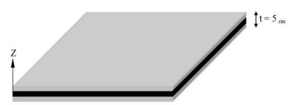
Figure 1. The square 3-layer composite plate
