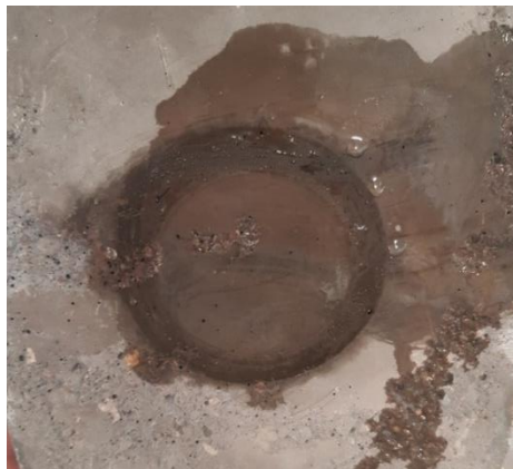
Figure 18 An image of a permeability sample after being removed from the test
