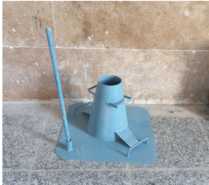
Figure 10. Slump test cone
