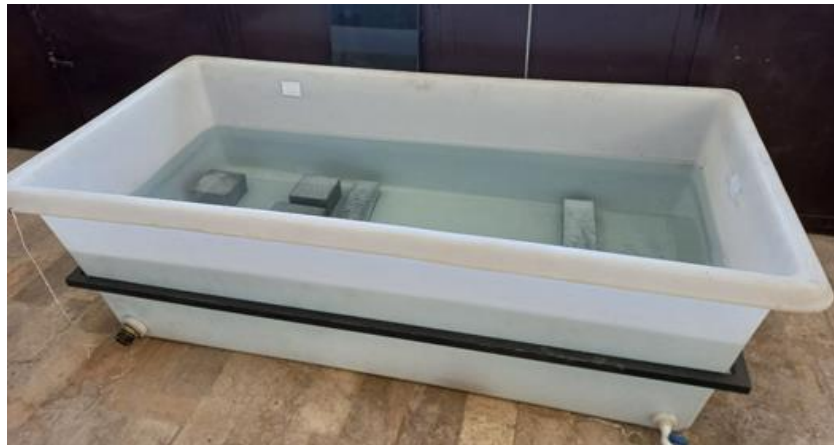
Figure 8. Concrete curing water bath
