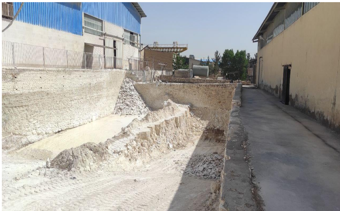
Figure 4. Gathering travertine sludge in the pools near stone processing plants
