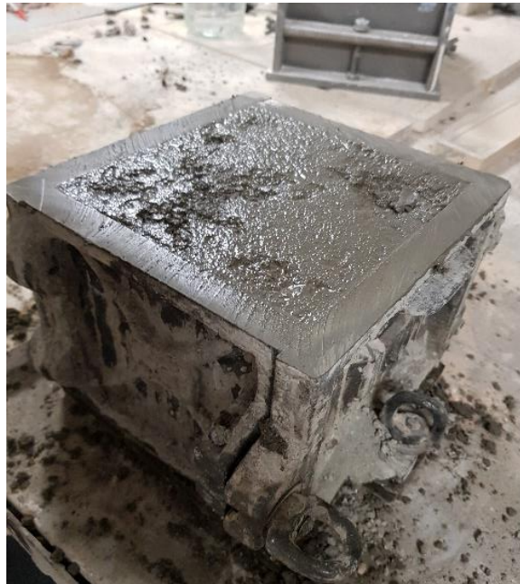
Figure 11. A 150 millimeter mold filled with concrete
