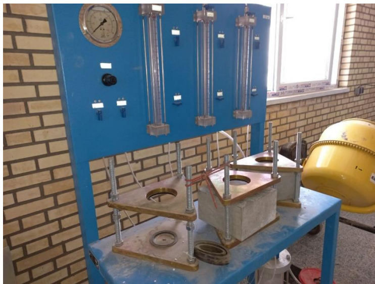
Figure 17 An image of the permeability test apparatus
