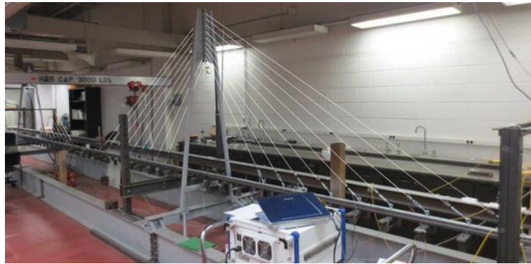
Figure 13: Laboratory Cable-Stayed Bridge [27]
