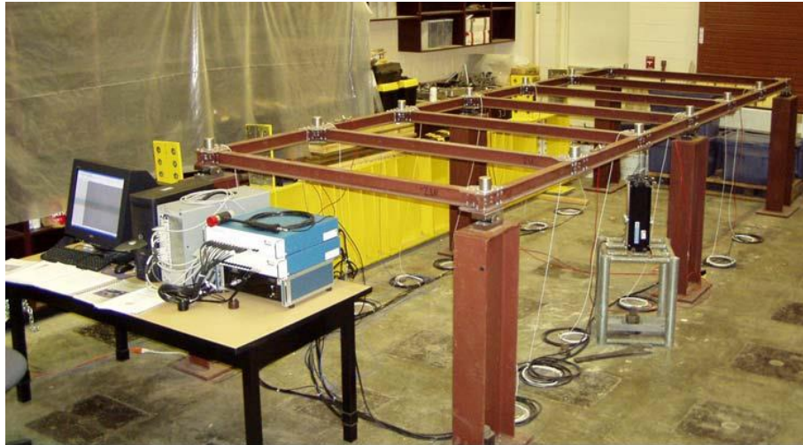
Figure 9: Two-Span Steel Grid benchmark [26]
