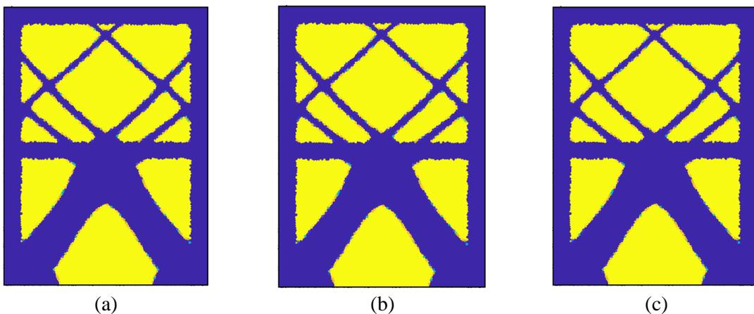
Figure 5. Optimized topologies obtained for the low-rise case using different earthquake ground motions: (a) Accelerogram 1, (b) Accelerogram 2, and (c) Accelerogram 3.
