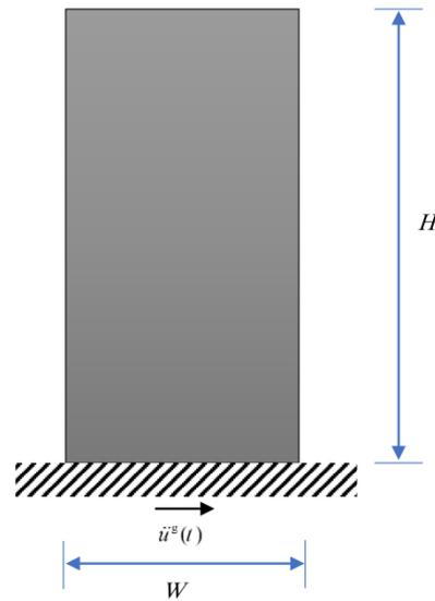
Figure 4. The ground structure used in topology optimization under a horizontal earthquake excitation.
