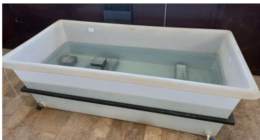
Figure 8. Concrete curing water bath
