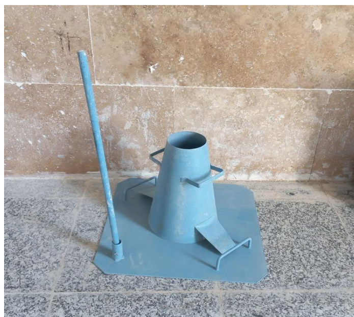
Figure 10. Slump test cone
