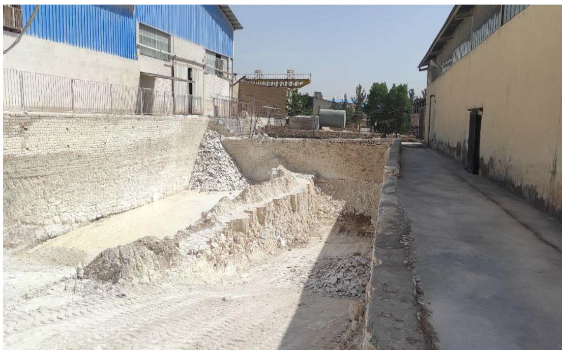
Figure 4. Gathering travertine sludge in the pools near stone processing plants
