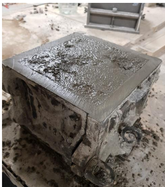
Figure 11. A 150 millimeter mold filled with concrete
