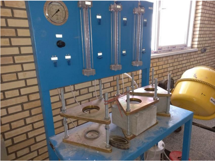
Figure 17 An image of the permeability test apparatus
