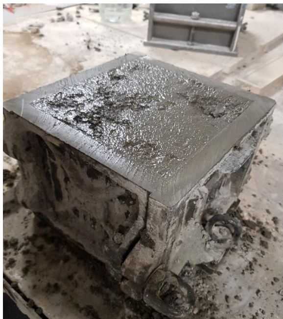
Figure 11. A 150 millimeter mold filled with concrete
